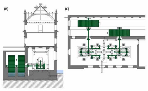
Fig. 4.215: Prague – pumping station of the Old Town Waterworks after reconstruction and modernisation in 1882. Machines from 1860 were replaced with four double-acting Girard pumps, which were powered by iron wheels with wooden blades. A – longitudinal section of the anti-freezing chamber, B – cross-section, C – ground plan (detail), 1 – water wheels, 2 – double-acting pumps. Diagram by Radek Míšanec, 2021 (modified according to: plan from APVK, the PVK photoarchive, kt. N 11, sig. B 013a/88).
