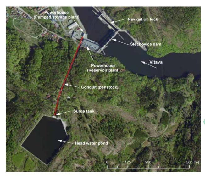
Fig. 4.162: Situation of the Štěchovice HS with a PSHPP and a HPP situated below the dam. Diagram created on the basis of the ČÚZK data, 2021.
