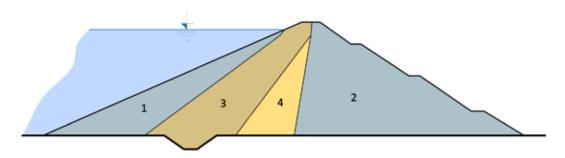
Fig. 4.30: Zoned earthfill dam: 1 – upstream shoulder from rubble, 2 – downstream shoulder from rubble, 3 – earth impervious zone, 4 – downstream shoulder from earth. Diagram by Radka Račoch, 2021 (modified according to: Broža et al., 2005).
