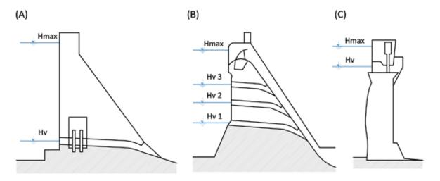
Fig. 4.47: Height position of outlets. (A) Bottom outlets; (B) Middle outlets; (C) Upper outlets. Diagram by Radka Račoch and Radek Bachan, 2021 (modified according to: Broža et al., 1987).
