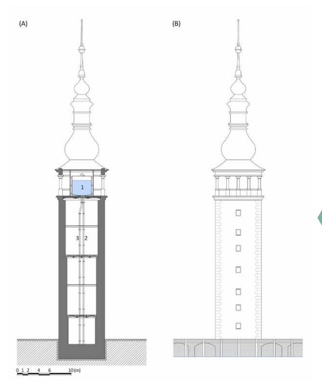
Fig. 4.213: Prague – The Old Town Water Tower was built for the purposes of the Old Town Waterworks. A – section, B – elevation, 1 – convex-bottom cylindrical tank, 2 – inlet pipeline, 3 – outlet pipeline. Diagram by Radek Míšanec, 2021 (modified according to: plan from APVK, unsign.).
