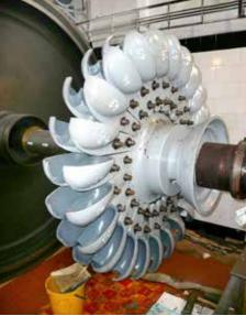
Fig. 4.203: Rudolfov I SHPP – twin horizontal Pelton turbine at the time of reconstruction. Photograph by Petr Freiwillig, 2012.
