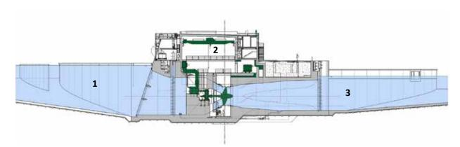
Fig. 4.151: Small hydroelectric power plant in Litoměřice – longitudinal section: 1 – inlet structure, 2 – machine room, 3 – outlet structure (taken from: Aquatis, a.s.).
