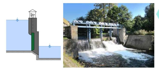
Fig. 4.132: On the left, a sluice (slide) lift weir. Diagram by Radka Račoch and Radek Bachan, 2021 (modified according to: Gabriel et al., 1989). On the right, a sluice gate weir on the Metuje River in Hronov (taken from: vodnimlyny.cz, 2013).
