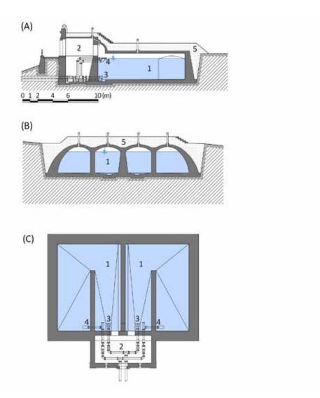
Fig. 4.237: Jičín – ground concrete water tank of a rectangular ground plan. A – cross-section, B – longitudinal section, C – ground plan, 1 – water tank compartment, 2 – valve chamber/control structure (building), 3 – inflow pipeline, 4 – outflow pipeline, 5 – earth embankment. Diagram by Radek Míšanec, 2021 (modified according to: Klír and Klokner, 1923).
