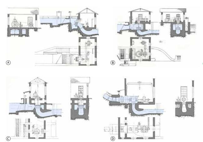
Fig. 4.201: Turbine water supply: (A) and (B) scroll case; (C) concrete spiral; (D) boiler water supply. Diagram by Radka Račoch, 2021 (modified according to: Nechleba, 1962)
