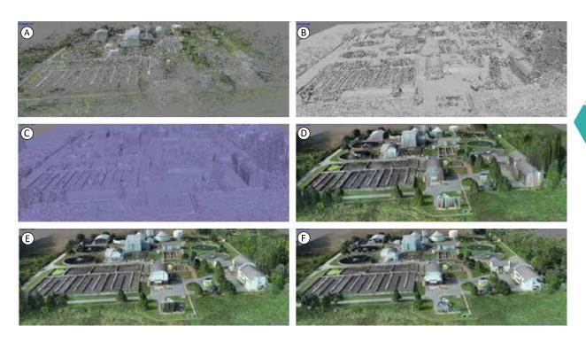
Fig. 4.296: Individual steps of the genesis of the 3D model of a large municipal WWTP: (A) identification of common points in individual photographs; (B) creation of point clouds; (E) creation of a wire model; (D) matching a colour scale of individual photograph to the 3D model; (E) model texturing; (F) final texture touches. Radek Bachan, 2021.
