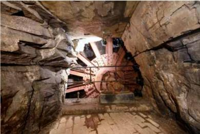
Fig. 4.190: Příbram, the Drkolnov mine – water wheel 12.4 m in diameter. Photograph by Viktor Mácha, 2019.
