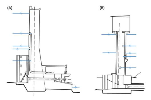
Fig. 4.58: Intake structures: (A) Multi-level intake structure in the dam body; (B) Multi-level tower intake structure. Diagram by Radka Račoch and Radek Bachan, 2021 (modified according to: Broža et al., 1987).
