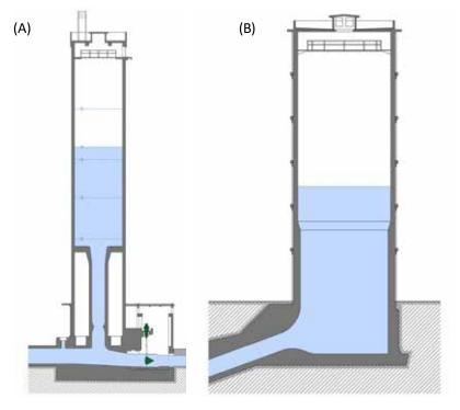
Fig. 4.181: Section of an overground surge chamber with diaphragm: (A) Práčov I SHPP; (B) Seč SHPP. Diagram by Radek Míšanec, 2021 (modified according to: Trejtnar, 1975).
