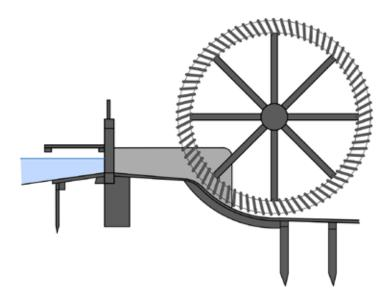
Fig. 4.193: Undershot water wheel with a masonry breast. Diagram by Radka Račoch and Michaela Mrvová, 2021 (modified according to Neumann, 1862).
