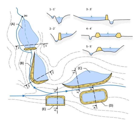
Fig. 4.71: Types of reservoirs without natural inflow and their cross-section: (A) – valley by-pass, (B) – bank, (C) – side, (D) – impound, (E) – dug. Diagram by Radka Račoch and Radek Bachan, 2021 (modified according to: Šálek, 1996).
