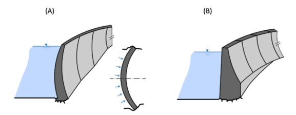
Fig. 4.44: (A) Arch dam; (B) Arch gravity dam. Diagram by Radka Račoch, 2021 (modified according to: Broža et al., 2005).
