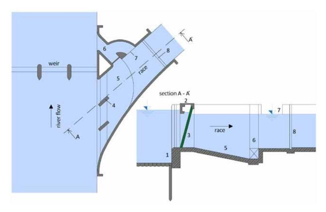
Fig. 4.166: Diagram of a derivation hydroelectric power plant inlet structure: 1 – intake sill, 2 – scumboard, 3 – coarse rack, 4 – dividing pier, 5 – settling tank, 6 – flushing channel, 7 – side (residual) overflow, 8 – regulating valve. Diagram by Radek Míšanec, 2021 (modified according to: Kratochvíl, 1956).
