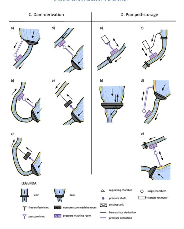
Fig. 4.148: Dam-derivation and pump schemes of hydropower works. Diagram by Radka Račoch and Michaela Mrvová, 2021 (modified according to Broža et al., 1990; Čábelka, 1958).
