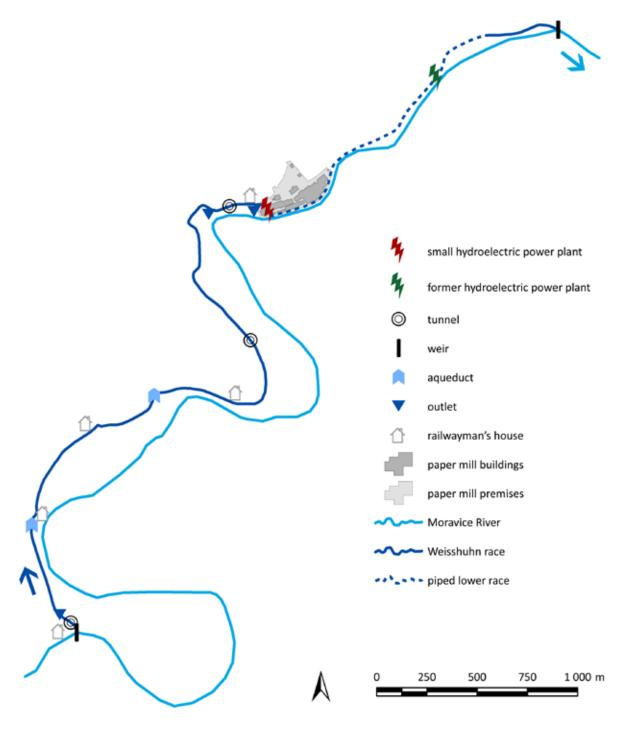
Fig. 4.206: Žimrovice – functional complex of the paper mill with individual important structures indicated. Diagram by Radek Míšanec, 2021 (modified according to: SOkA Opava, karton 1052, 1911–1914).
