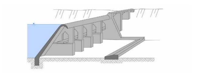
Fig. 4.127: Multiple buttress weir. Diagram by Radek Míšanec, 2021 (modified according to: Gabriel et al., 1989).
