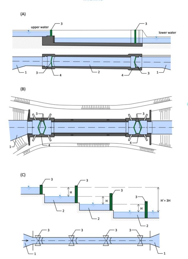
Fig. 4.101: (A) Diagram of a simple lock chamber; (B) Lock with double gates; (C) Diagram of a multi-level lock chamber; 1 – lock cut, 2 – the lock chamber itself, 3 – lock chamber gates, 4 – head. Diagram by Radka Račoch and Michaela Mrvová, 2021 (modified according to: VSB – Technical University of Ostrava, 2013).
