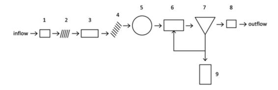
Fig. 4.258: A block diagram of a WWTP technological line: 1 – gravel trap, 2 – screen, 3 – sand and grease trap, 4 – lift station, 5 – settling tank, 6 – biological reactor, 7 – secondary settling tank, 8 – tertiary treatment, 9 – sludge handling and disposal. Diagram by Radka Račoch and Radek Bachan, 2021 (modified according to: the TGM WRI archive).
