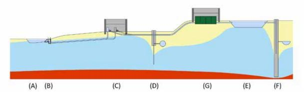
Fig. 4.227: Káraný, Káraný waterworks – diagram of water treatment: (A) weir on a lake; (B) intake structure; (C) raw water pumping station; (D) drilled wells; (E) drop caissons with horizontal collectors; (F) infiltration tanks; (G) water treatment plant with rapid sand filter, infiltration tanks. Diagram by Radek Míšanec, 2021 (modified according to: diagram of the Prague Waterworks Museum).
