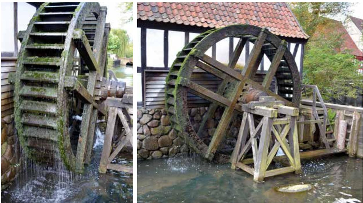
Fig. 4.192: Undershot water wheel with floats and shrouds, but without sole boards, which has incomplete buckets. Photograph by Radim Urbánek, 2015.
