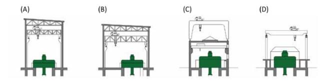
Fig. 4.182: Types of upper machine building layout: (A) and (B) covered; (C) semi-covered; (D) uncovered – without the upper structure. Diagram by Radek Míšanec, 2021 (modified according to: Hodák, 1998).
