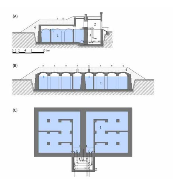
Fig. 4.236: Prague-Vršovice – ground water tank in Zelená Liška (part of Vršovice waterworks), an example of ground brick water tank. A – cross-section, B – longitudinal section, C – ground plan, 1 – water tank compartment/water tank meander chamber, 2 – valve chamber/control structure (building), 3 – inflow and outflow pipeline, 4 – earth embankment. Diagram by Radek Míšanec, 2021 (modified according to: Klír and Klokner, 1923).
