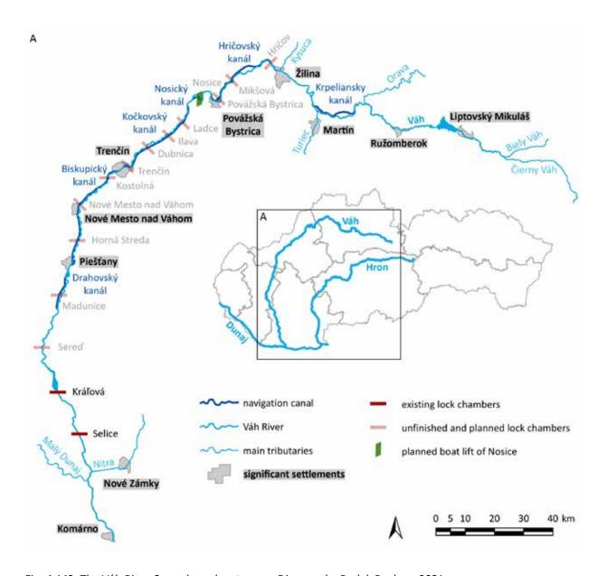
Fig. 4.142: The Váh River Cascade and waterway. Diagram by Radek Bachan, 2021.
