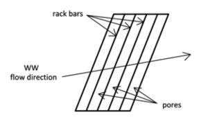
Fig. 4.261: Description of individual screen parts. Diagram by Radka Račoch and Radek Bachan, 2021 (modified according to: the TGM WRI archive).
