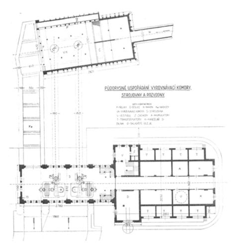
Fig. 4.180: Surge chamber layout, supply pressure pipeline and machine room of the Spálov SHPP (taken from: ZSV, 1924)
