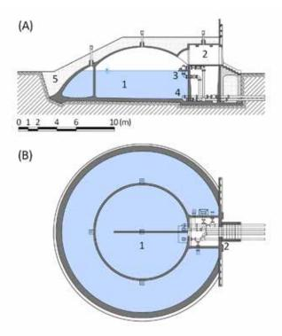
Fig. 4.238: Ground reinforced concrete water tank of a spherical shape. A – cross-section, B – ground plan, 1 – water tank compartment, 2 – valve chamber/control structure (building), 3 – inflow pipeline, 4 – outflow pipeline, 5 – earth embankment. Diagram by Radek Míšanec, 2021 (modified according to: Klír and Klokner, 1923).
