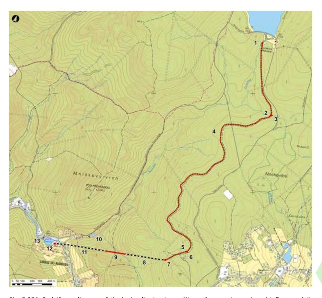
Fig. 5.304: Rudolfov – diagram of the hydraulic structures: (1) small measuring weir and inflow conduit, (2) 1. aqueduct, (3) 1. tank, (4) underground conduit, (5) 2. aqueduct, (6) 2. tank, (7) water cutoff, (8) pressure pipeline, (9) overground section on pillars, (10) gravel obstruction with a cistern, (11) pressure pipeline, (12) peaking power plant, (13) run-of-river power plant (taken from: Freiwillig, 2019).
