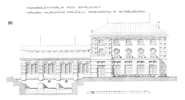
Fig. 4.176: Spálov SHPP: (A) longitudinal section of a surge chamber, supply pressure pipeline and machine room; (B) view of the machine room and surge chamber at the end of the headrace (taken from: VČE, 2000). Continued from previouse page.
