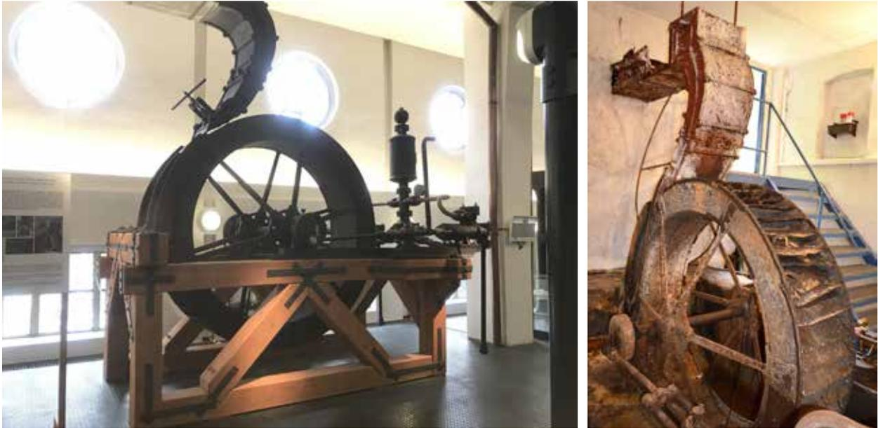
*Fig. 4.224: Pavlovice u České Lípy – local waterworks was built and the machinery produced by the J. Gater – Hühnerwasser company in 1902, when a collecting structure of potable water and a pumping station were built and the flow of Dolský Brook modified. The pumping and water transport was ensured by a horizontal double-acting pump powered by an overshot waterwheel, the so-called Gatter wheel. The original pumping set worked until the mid-1970s. Photograph from the PVK archive, 2010 and 2018.*
