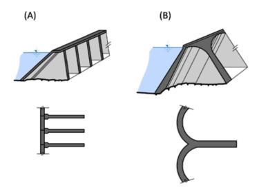
Fig. 4.46: (A) Flat-slab multiple dam; (B) Dome multiple dam. Diagram by Radka Račoch, 2021 (modified according to: Broža et al., 2005).
