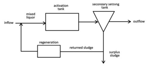
Fig. 4.274: A block diagram of regenerating activation. Diagram by Radka Račoch and Radek Bachan, 2021 (modified according to: the TGM WRI archive).
