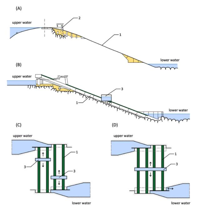
Fig. 4.105: Inclined plane lifts: (A) Rail transport of smaller boats on a cart; (B) Rail transport of larger vessels in a straight movable trough; (C) Transverse movable trough, dual rail track; (D) Possibility of connecting two troughs for the transport of long boats; 1 – rail track, 2 – cart for transporting small boats, 3 – movable trough for transporting larger vessels. Diagram by Radka Račoch and Michaela Mrvová, 2021 (modified according to: Březinský, 2020 and VSB – TUO, 2013)
