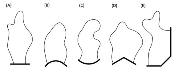
Fig. 4.73: Dam front shapes: (A) straight; (B) convex; (C) concave; (D) polygonal; (E) irregular. Diagram by Radka Račoch and Radek Bachan, 2021 (modified according to: Šálek, 1996).
