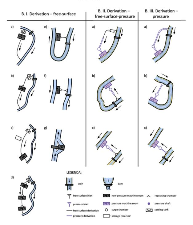
Fig. 4.147: Derivation schemes of hydropower works. Diagram by Radka Račoch and Radek Bachan, 2021 (modified according to: Broža et al., 1990; Čábelka, 1958).
