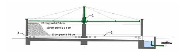
Fig. 4.272: Section of the most common type of biofilter: 1 – rotating sprinkler, 2 – permeable grid, 3 – ventilation openings, inside the structure – filter medium (sand, gravel, composition of various fractions), the picture shows an example of a basic composition of a filter medium with diameters of material grains (fractions). Diagram by Radka Račoch and Michaela Mrvová, 2021.
