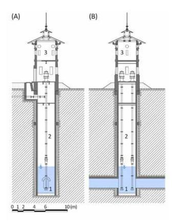
Fig. 4.229: Benešov near Prague – tube well with a pumping station. A – cross-section, B – longitudinal section, 1 – suction strainers, 2 – pumping pipeline, 3 – pumping station building. Diagram by Radek Míšanec, 2021 (modified according to: Klír and Klokner, 1923).
