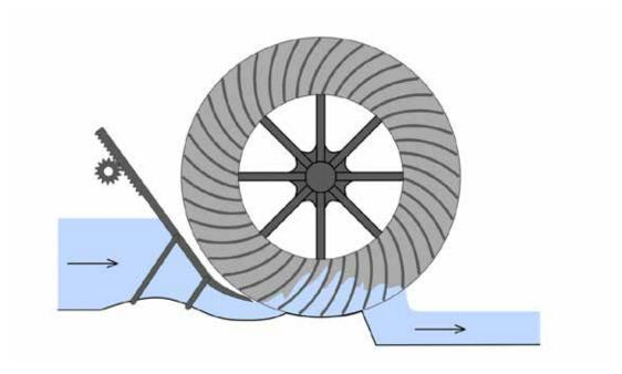
Fig. 4.194: Poncelet water wheel. Diagram by Radka Račoch and Michaela Mrvová, 2021 (modified according to Hýbl 1922; Štěpán et al., 2008; NM, 2021).
