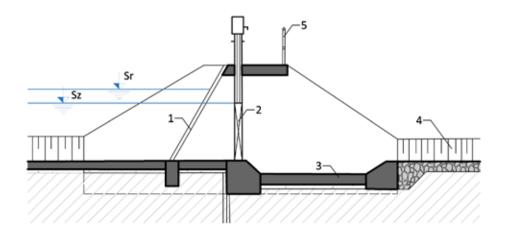
Fig. 4.81: Diagram of a sluice gate: 1 – rack, 2 – sluice gate, 3 – stilling basin, 4 – tailrace, 5 – operation bridge, Sz – level of storage area, Sr – level of controllable retention area. Diagram by Radka Račoch and Michaela Mrvová, 2021 (modified according to Tlapák, Herynek, 2002).
