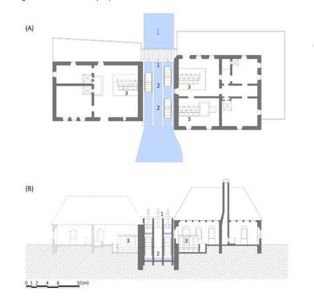
Fig. 4.205: Brno-Husovice – fulling mill, reconstruction of the state at the end of the 18th century. A – ground plan, B – longitudinal section, 1 – sluice gate, 2 – water wheel, 3 – fulling mill facilities. Diagram by Radek Míšanec, 2018 (according to: Freudenberger, 1977).
