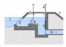
Fig. 4.233: Riverside intake: 1 – watercourse, 2 – rack, 3 – scumboard, 4 – measuring sill, 5 – shaft, 6 – sluice gate, 7 – dam, 8 – water intake piping. Diagram by Radek Míšanec, 2021 (modified according to: Milerski 2005).
