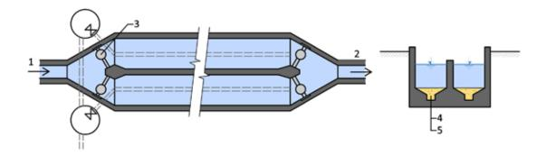
Fig. 4.264: Chamber sand trap: 1 – inflow, 2 – outflow, 3 – sluice gate, 4 – sedimented material, 5 – drainage. Diagram by Radka Račoch and Radek Bachan, 2021 (modified according to: the TGM WRI archive).
