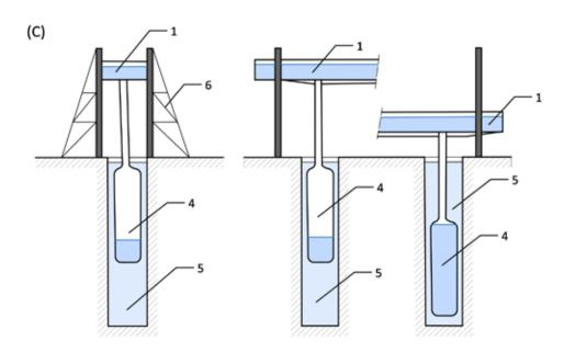
Fig. 4.104: Vertical boat lifts: (A) Piston boat lift; (B) Diagram of a boat lift with counterweights; (C) Diagram of a boat lift with floats; 1 — basin for boat transport; 2 — hydraulic-controlled piston; 3 — counterweight; 4 — float, 5 — solid technological elements, 6 — overground supporting structure. Diagram by Radka Račoch and Michaela Mrvová, 2021 (modified according to: VSB – Technical University of Ostrava, 2013).
