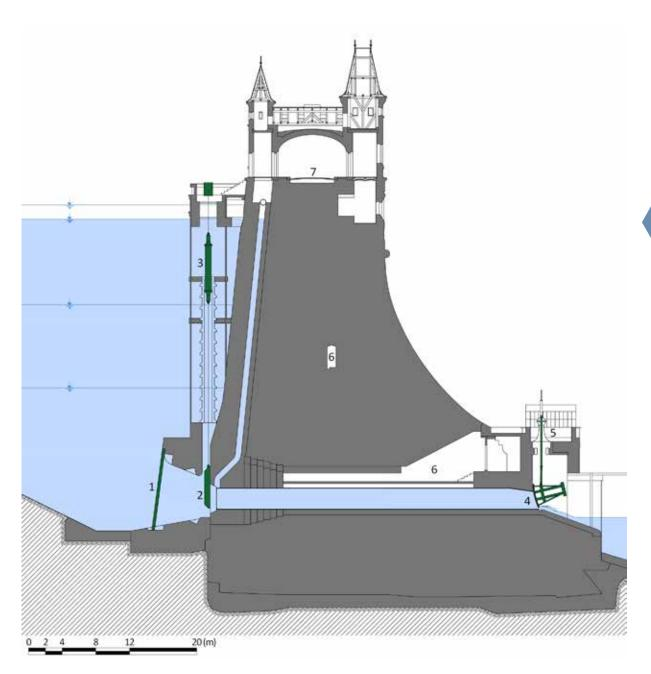
Fig. 4.64: The Les Království dam (1910–1919) – cross-section of the dam at the bottom outlet: 1 – thrashracks, 2 – gate valve, 3 – control of the gate valve, 4 – radial gate valve, 5 – control of the radial gate valve, 6 – inspection gallery, 7 – crest of the dam. Diagram by Radek Míšanec, 2021 (adapted according to: the Elbe River basin archive).
