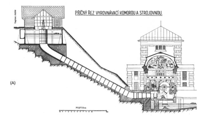
Fig. 4.176: Spálov SHPP: (A) longitudinal section of a surge chamber, supply pressure pipeline and machine room; (B) view of the machine room and surge chamber at the end of the headrace (taken from: VČE, 2000).
