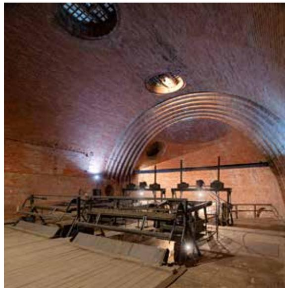
*Fig. 3.24: Prague-Bubeneč, old wastewater treatment plant. This treatment plant, designed by William H. Lindley in 1894, is one of the most important European examples of a solution to the problem of wastewater – an issue faced by rapidly growing industrial cities towards the end of the 19th century. For more information see Chapter 4.6. Drainage/sewerage and wastewater treatment. Photograph by Viktor Mácha, 2020.*
