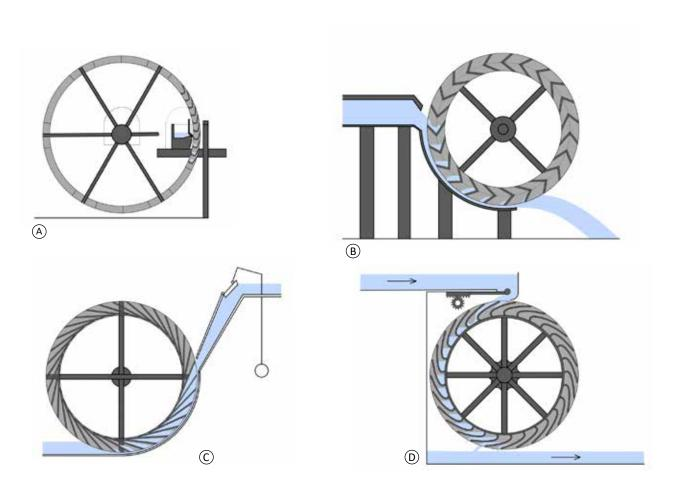
Fig. 4.188: Bucket water wheels: (A) breastshot water wheel with inner inflow, i.e., with inner buckets; (B) breastshot or overshot water wheel (water level above shaft level) with a masonry breast; (C) reverse overshot water wheel – older type on the left, newer type with rounded buckets on the right. Diagram by Radka Račoch and Michaela Mrvová, 2021 (modified according to: Hýbl 1922, 1862; Štěpán, 1990; Štěpán and Křivanová, 2000).
