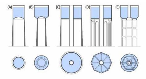
Fig. 4.240: Examples of construction solutions of water tanks with reinforced concrete structure. (A) cylindrical below the perimeter of the cistern, (B) cylindrical on a foundation wall (Intze-type), (C) cylindrical, peripheral and shaft on a double foundation wall, (D) on radial walls – solid or with openings, (E) on several pillars. Diagram by Radek Míšanec, 2021 (modified according to: Klír and Klokner, 1923).
