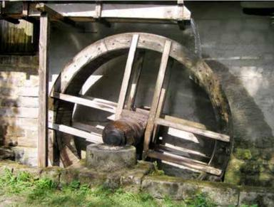
Fig. 4.189: Overshot bucket water wheel. Photograph by Radim Urbánek, 2006.
