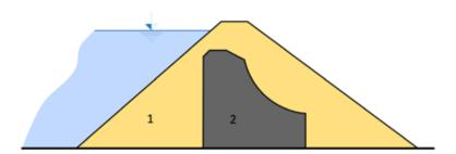
Fig. 4.40: Composite dam: 1 – earthfill part, 2 – gravity part from concrete. Diagram by Radka Račoch and Radek Bachan, 2021 (modified according to: Broža et al., 1987).
