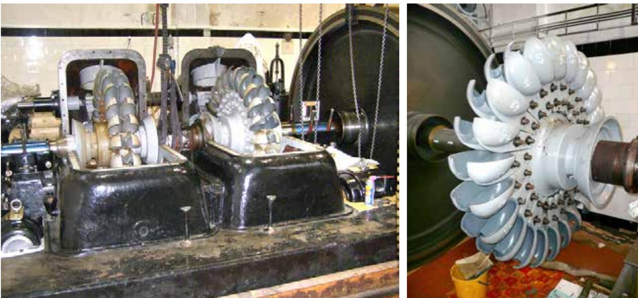
*Fig. 4.203: Rudolfov I SHPP – twin horizontal Pelton turbine at the time of reconstruction. Photograph by Petr Freiwillich, 2012.*
