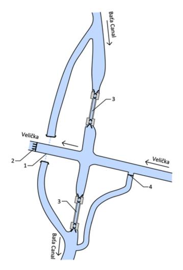
Fig. 4.110: Diagram of the crossing of the Baťa Canal and the Velička River: 1 - inverted siphon to maintain the same water level of the navigable canal, 2 - weir regulating the water level of the Velička River, 3 - lock chambers with double gates, 4 - sluice gate. Diagram by Radka Račoch and Radek Bachan, 2021 (modified according to the situation in the terrain in 2020).
