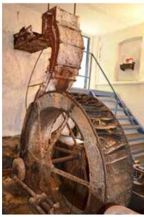
Fig. 4.224: Pavlovice u České Lípy – local waterworks was built and the machinery produced by the J. Gater – Hühnerwwasser company in 1902, when a collecting structure of potable water and a pumping station were built and the flow of Dolský Brook modified. The pumping and water transport was ensured by a horizontal double-acting pump powered by an overshot waterwheel, the so-called Gatter wheel. The original pumping set worked until the mid-1970s. Photograph from the PVK archive, 2010 and 2018.
