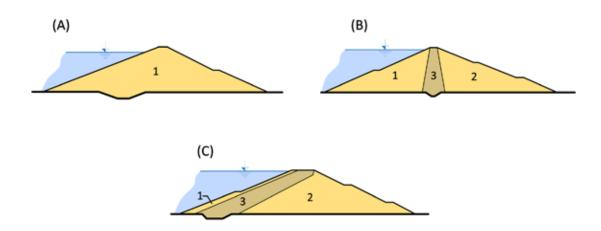
Fig. 4.28: Basic types of earthfill dams: (A) Earthfill homogeneous: 1 — stabilising part (shoulder); (B) Earthfill with hearting zone: 1 — upstream shoulder, 2 — downstream shoulder, 3 — earth seal (core); (C) Earthfill with inclined upstream impervious zone: 1 — revetment, 2 — downstream shoulder, 3 — earth upstream impervious zone. Diagram by Radka Račoch, 2021 (modified according to: Broža et al., 2005).
