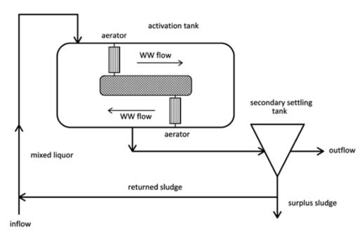
Fig. 4.275: Oxidation ditch. Diagram by Radka Račoch and Radek Bachan, 2021 (modified according to: the TGM WRI archive).
