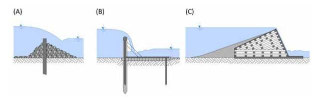
Fig. 4.122: Types of timber weirs: (A) A damming structure with timber pile wall complemented by stabilising stone material; (B) A damming structure stabilised by timber struts; (C) A crib weir structure. Diagram by Radek Míšanec, 2021 (modified according to: Průcha, 1980).
