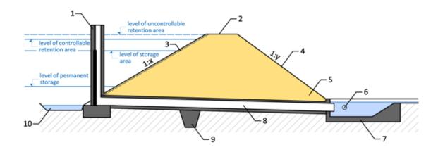
Fig. 4.67: General reservoir scheme: (1) – outlet structure (monk outlet), (2) – dam crest, (3) – upstream face, (4) – downstream face, (5) – toe drain, (6) – pipeline pit, (7) – stilling basin, (8) – outlet pipeline, (9) – cutoff, (10) – dead storage. Diagram by Radka Račoch and Radek Bachan, 2021 (modified according to: Ministry of Agriculture, 2015).
