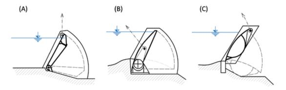
Fig. 4.130: Types of flap gates: (A) panel; (B) pipe; (C) hollow. Diagram by Radka Račoch and Michaela Mrvová, 2021 (modified according to Průcha, 1980).
