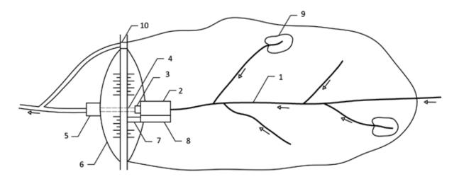
Fig. 4.93: Diagram of a fishpond with structures and specially prepared bottom: 1 – main drainage sewer, 2 – fishing ground, 3 – monk outlet, 4 – pipeline, 5 – stilling basin, 6 – dam, 7 – access stairs, 8 – space for tubs, 9 – drainage of gutters, 10 – safety spillway. Diagram by Radka Račoch and Radek Bachan, 2021 (modified according to: Pokorný, 2009).
