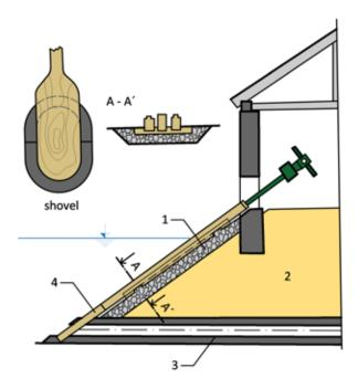
Fig. 4.83: Shovel valve: 1 – stone riprap, 2 – dam body, 3 – bottom outlet, 4 – bottom part of the blade. Diagram by Radka Račoch and Michaela Mrvová, 2021 (modified according to Vrána, Beran, 2008).
