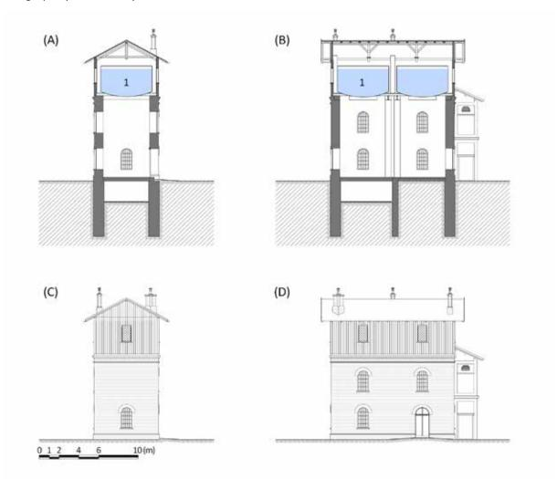
Fig. 4.248: Skalice nad Svitavou – railway elevated water tank with two cylindrical tanks, built according to the standardised project by C. k. ředitelství pro tratě of the former Společnost státní dráhy from 1910. An example of the use of an elevated water tank for other than water supply purposes. A – cross-section, B – longitudinal section, C, D – elevations, 1 – convex-bottom cylindrical tank. Diagram by Radek Míšanec, 2018 (modified according to: plan documentation).
