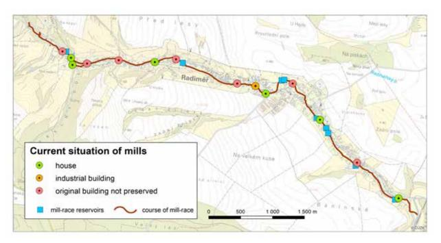
Fig. 3.5: System of the Radiměř mill-race, with 14 mills and 9 small hydroelectric power plants – current situation (the course of the mill-race has partially survived as a landscape remnant); an example of a wider-ranging
