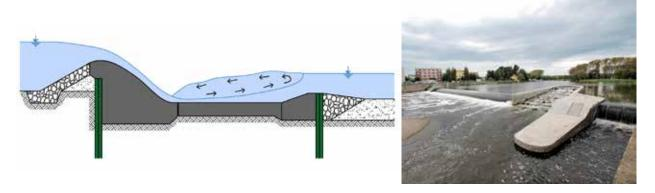
Fig. 4.126: On the left, a fixed concrete weir. Diagram by Radka Račoch and Radek Bachan, 2021 (modified according to: Gabriel et al., 1989). On the right, a weir in Břeclav. Photograph from the Brno University of Technology archive, 2019.
