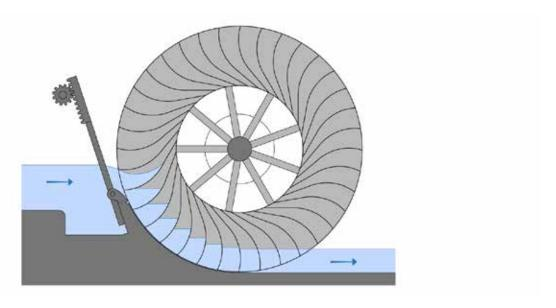
Fig. 4.196: Zuppinger water wheel. Diagram by Radek Míšanec, 2021 (modified according to: Hýbl 1922).
