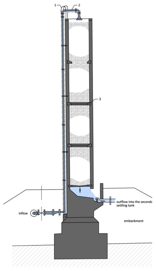
Fig. 4.271: Tower biofilter: 1 – steel ladder, 2 – thermally isolated pipeline for the purified water intake, 3 – buffle, inside the structure – filter medium (sand, gravel, composition of various fractions). Diagram by Radka Račoch and Michaela Mrvová, 2021.
