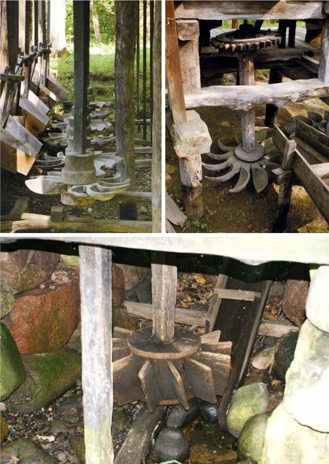
*Fig. 4.197: Horizontal water wheel. Photograph by Radim Urbánek, 2011.*
