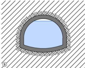
Fig. 4.174: Spálov SHPP – free-surface gallery: (A) view of the gallery after reconstruction with the use of geomembrane. Photograph taken from: VČE, 2000; (B) diagram by Radek Míšanec, 2021 (modified according to: ZČE, 2000).
