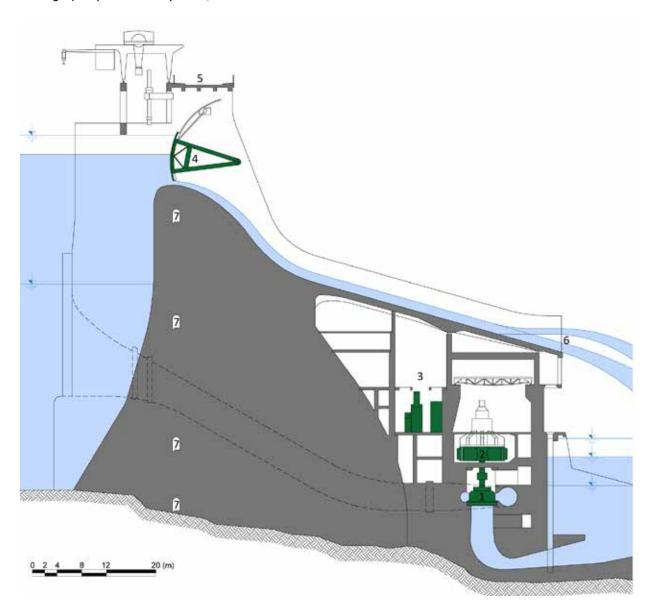
Fig. 4.157: Slapy HPP adjacent to the dam situated under the spillway: 1 – Kaplan turbine, 2 – generator, 3 – switch house, 4 – safety spillway radial gate, 5 – bridge deck, 6 – chute ending with baffle blocks, 7 – concrete gravity dam. Diagram by Radek Míšanec, 2021 (modified according to: Štoll, 1977).
