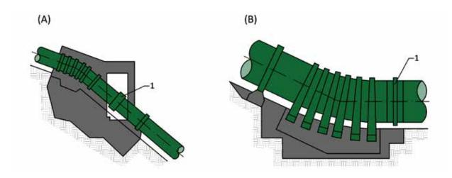
Fig. 4.179: Examples of anchor blocks construction: (A) closed type; (B) open type; 1 – compensation pipe. Diagram by Radka Račoch and Radek Bachan, 2021 (modified according to: Broža et al., 1990).
