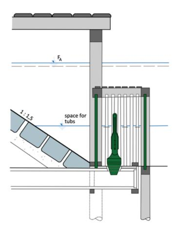
Fig. 4.82: Pin valve:  $F_A$  – maximum water level. Diagram by Radka Račoch and Michaela Mrvová, 2021 (modified according to Pavelková et al., 2014).
