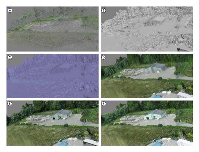
Fig. 4.294: Individual steps of the genesis of the 3D model of a small WWTP: (A) identification of common points in individual photographs; (B) creation of point clouds; (E) creation of a wire model; (D) matching a colour scale of individual photograph to the 3D model; (E) model texturing; (F) final texture touches. Radek Bachan, 2021.
