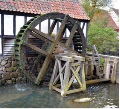
Fig. 4.192: Undershot water wheel with floats and shrouds, but without sole boards, which has incomplete buckets. Photograph by Radim Urbánek, 2015.
