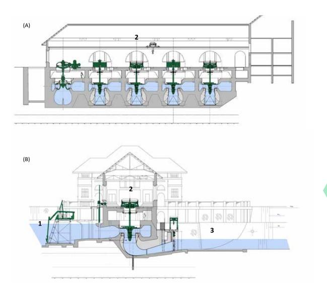
Fig. 4.150: Small hydroelectric power plant in Miřejovice on a short (A) cross-section, (B) longitudinal section 1 – inlet structure, 2 – machine room, 3 – outlet structure (taken from: Aquatis, a.s.).
