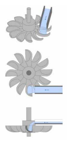
Fig. 4.198: Horizontal water wheel. Diagram by Radek Míšanec, 2021 (modified according to: Zeising, 1612).
