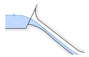
Fig. 4.57: Tunnel safety spillway. Diagram by Radka Račoch and Radek Bachan, 2021 (modified according to: Broža et al., 1987).
