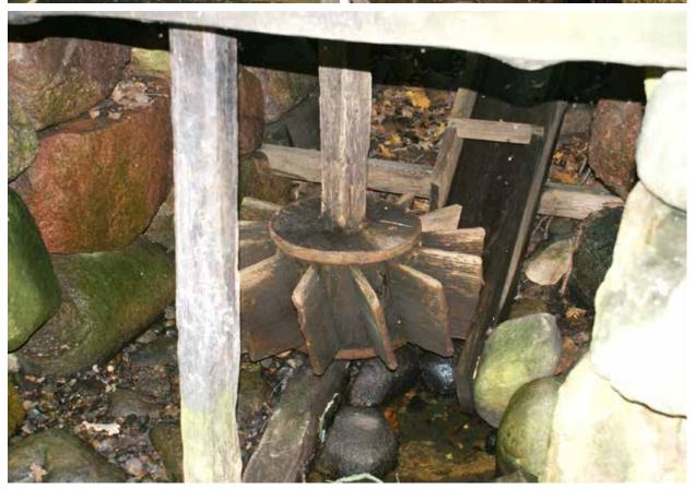
Fig. 4.197: Horizontal water wheel. Photograph by Radim Urbánek, 2011.
