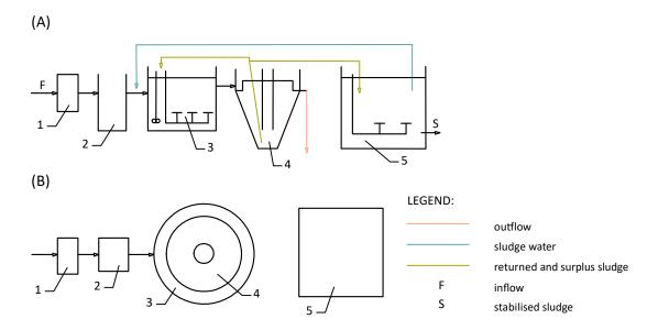
Fig. 4.291: An example of a model technology line of a standardised WWTP: 1 – coarse pre-treatment (screen), 2 – vertical sand trap, 3 – activation tank, simultaneous operation, 4 – nitrification and denitrification tank, 5 – vertical secondary settling tank, another structure outside the scheme – aerated sludge box. Diagram by Radka Račoch and Michaela Mrvová, 2021 (modified according to: provided project documentation).
