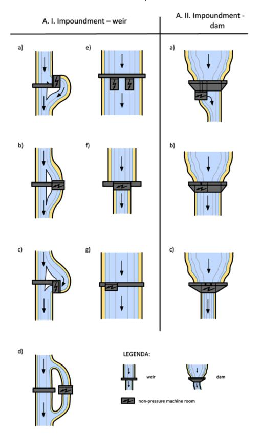
Fig. 4.146: Impoundment scheme of hydropower works. Diagram by Radka Račoch and Radek Bachan, 2021 (modified according to: Broža et al., 1990; Čábelka, 1958).
