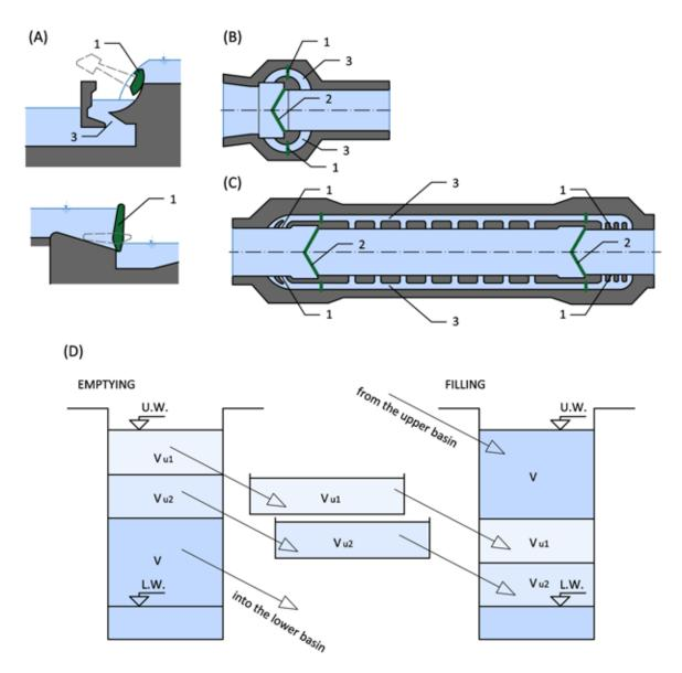
Fig. 4.102: Diagram of a lock chamber filling and emptying: (A) Filling by gates; (B) Filling by culverts of gates; (C) With filling openings along the entire length of the lock chamber; 1 – valve of the filling openings, 2 – gates of the lock chamber, 3 – filling and by-pass openings; (D) Thrift lock. Diagram by Radka Račoch and Radek Bachan, 2021 (modified according to: VSB – Technical University of Ostrava, 2013, (D) according to Moravová, 2020).
