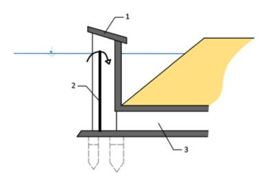
Fig. 4.84: General diagram – open monk outlet: 1 – crown of monk outlet with lockable lid, 2 – sluice wall, 3 – pipeline. Diagram by Radka Račoch and Radek Bachan, 2021 (modified according to: Slavík, Neruda, 2007).
