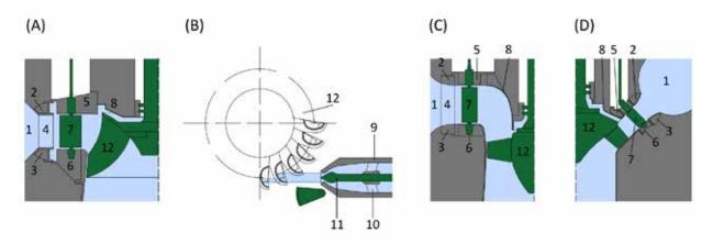
Fig. 4.199: Modern turbine solution diagrams: (A) Francis turbine; (B) Pelton turbine; (C) Kaplan turbine; (D) Deriaz turbine; 1 — spiral, 2 – upper stationary ring, 3 – lower stationary ring, 4 – stationary blade, 5 – upper blade ring, 6 – lower blade ring, 7 – guide vane, 8 – turbine lid, 9 – nozzle, 10 – guide blade, 11 – regulating needle, 12 – runner. Diagram by Radek Míšanec, 2021 (modified according to: Bednář, 1989).
