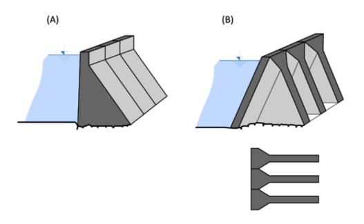
Fig. 4.42: (A) Gravity dam; (B) Buttress gravity dam. Diagram by Radka Račoch, 2021 (modified according to: Broža et al., 2005).
