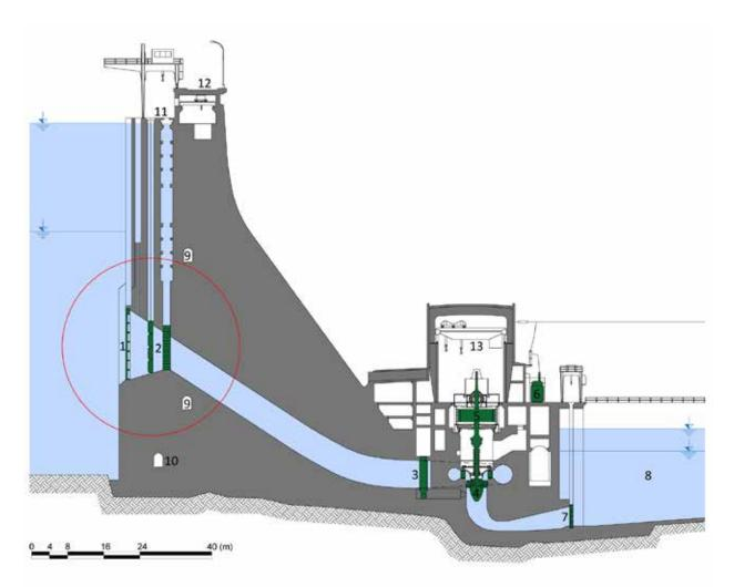
Fig. 4.169: Orlík HS – longitudinal section of the power plant block: 1 - rack, 2 - inspection and operational gates, 3 - operational gate in front of the turbine, 4 - Kaplan turbine, 5 - generator, 6 - block transformer, 7 - draught tube temporary flashboard, 8 - outlet structure, 9, 10 - inspection gallery, 11 - gantry crane, 12 - dam crest, 13 - upper machine building of the HPP. Diagram by Radek Míšanec, 2021 (modified according to: the Povodí Vltavy [Vltava River Basin] company archive).
