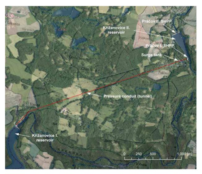
Fig. 4.161: Dam-derivation situation of the Práčov I SHPP and the Práčov II SHPP situated below the dam. Diagram created on the basis of the ČÚZK data, 2021.
