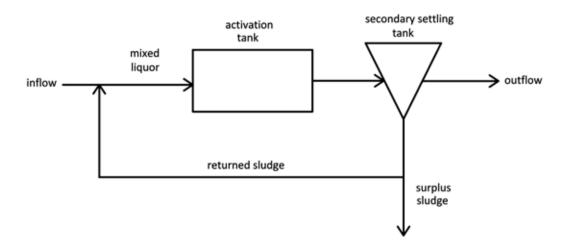
Fig. 4.273: A block diagram of classical activation. Diagram by Radka Račoch and Radek Bachan, 2021 (modified according to: the TGM WRI archive).
