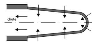
Fig. 4.56: Channel safety spillway. Diagram by Radka Račoch and Radek Bachan, 2021 (modified according to: Broža et al., 1987).
