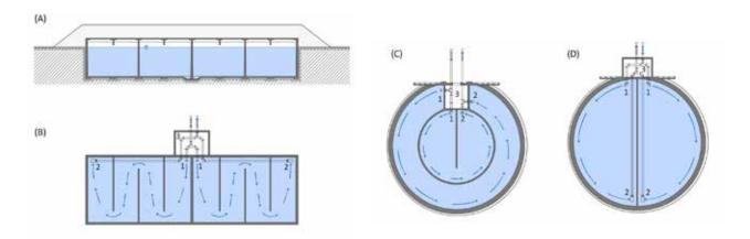
Fig. 4.235: Square and circular ground water tank. A – square ground water tank, longitudinal section, B – square ground water tank, ground plan, C, D – circular ground water tank with two compartments, ground plan, 1 – inflow pipeline, 2 – outflow pipeline, 3 – valve chamber/control structure (building). Diagram by Radek Míšanec, 2021 (modified according to: Klír and Klokner, 1923).
