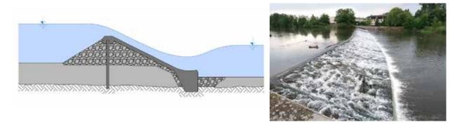
Fig. 4.124: On the left, a stone weir. Diagram by Radek Míšanec, 2021 (modified according to: Gabriel et al., 1989); on the right, a weir near Oblekovice. Photograph by Miriam Dzuráková, 2021.
