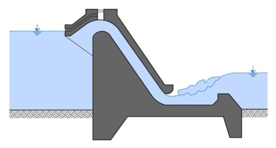
Fig. 4.128: Siphon weir. Diagram by Radka Račoch and Radek Bachan, 2021 (modified according to: Průcha, 1980).
