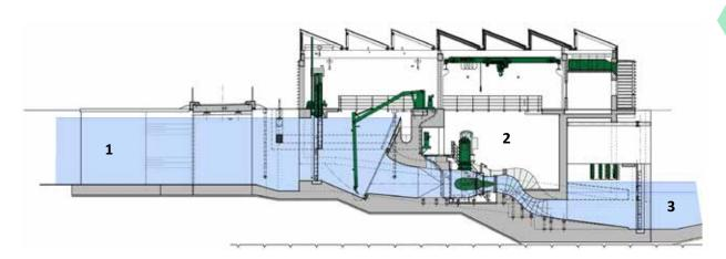
Fig. 4.160: Železný Brod SHPP – longitudinal section of the SHPP machine room in the turbine axis: 1 – inlet structure, 2 – machine room, 3 – outlet structure (taken from: Aquatis, a.s.).
