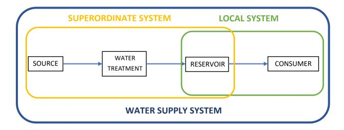
Fig. 4.251: Diagram of the whole water supply system – basic elements and classification. Diagram by David Honek, 2021.
