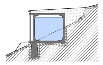
Fig. 4.172: Spálov SHPP – section of a reinforced concrete supply channel. Diagram by Radek Míšanec, 2021 (modified according to: ZSV, 1924).
