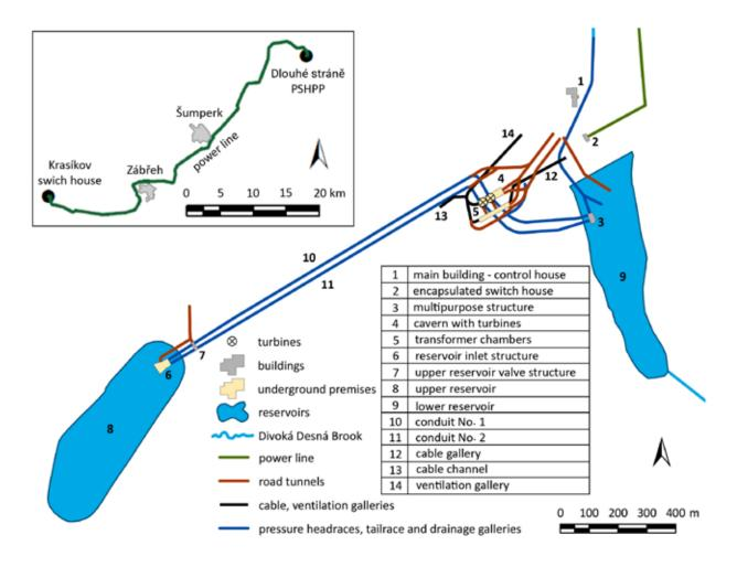
Fig. 4.208: Dlouhé stráně PSHPP – an overview map, including extra high voltage line. Diagram by Radek Míšanec, 2021 (modified according to: Kopřiva et al. 1997; ZAO – SOkA Šumperk, Dlouhé stráně PSHPP – overall solution of the construction; RUIAN [Registry of Territorial Identification, Addresses and Real Estate]; ZABAGED [Fundamental Base of Geographic Data of the Czech Republic]).
