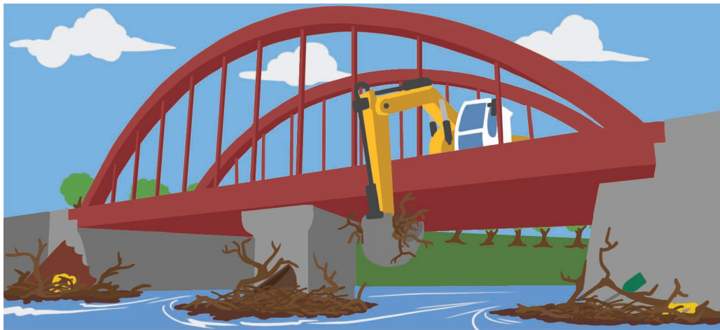
Removal of trapped floating debris
