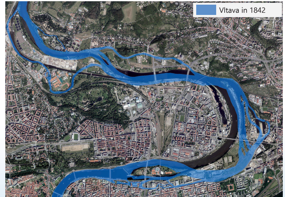
Channelization of the Vltava River at the turn of the 19th and 20th centuries determined its present form
