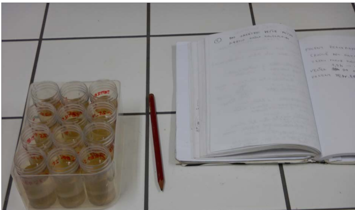
Fig. 87. Micromethod in test tubes (individual juvenile mussels breeds) with fewer space requirements and less need for detritus in the sample.
