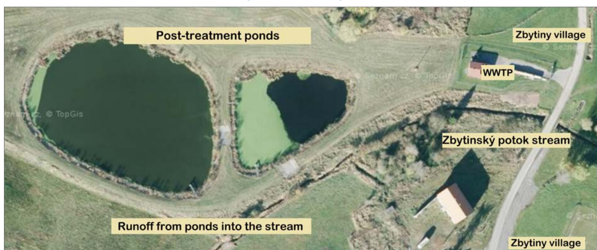
Fig. 250. Wastewater treatment system in the village of Zbytiny with post-treatment ponds. Source: Mapy.cz, © Seznam.cz, a. s., © TopGis, s. r. o.
