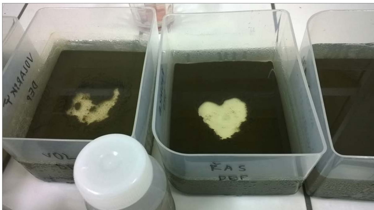
Fig. 90. Detritus for bioindications must be kept at a low temperature and samples carefully pipetted from the bottom of the container.
