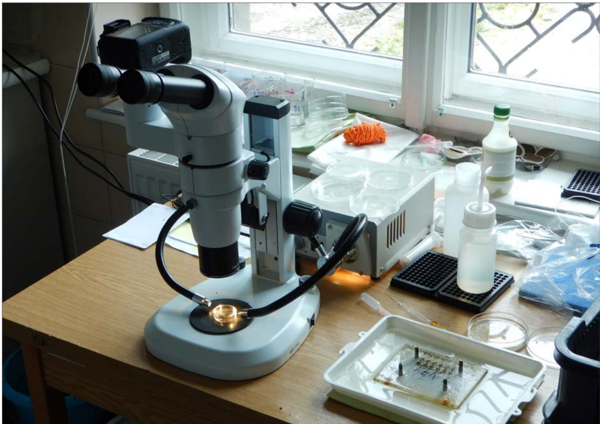
Fig. 70. Trinocular stereomicroscope equipped with a camera to take photographs of juvenile FPM.
