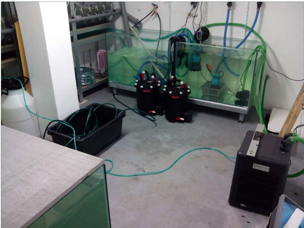
Fig. 49. Fish rearing facility. A recirculation rearing system made by K. Douda as a part of the EU project “Coexistence of humans and pearl mussels in the Vltava floodplain”, used by Šumava National Park Administration for FPM rearing.
