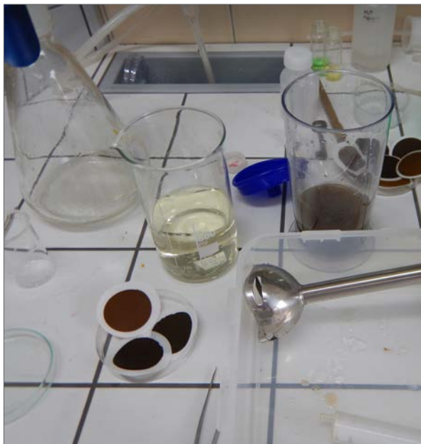
Fig. 29. Preparation of artificial analogues of detritus in the laboratory. On the far left a filtration device, natural water for dilution in a beaker, at the bottom GF/C filters with a fixed fraction after filtration of the homogenate and a stainless steel bar mixer.
