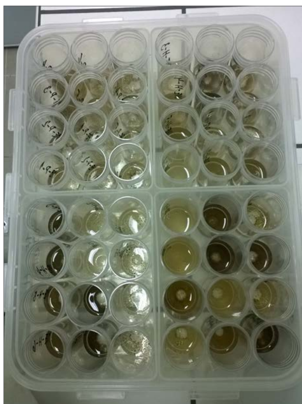
Fig. 88. Micromethod of laboratory bioindications in test tubes. The large food storage box can hold up to 48 test tubes for individual exposure of juvenile mussels.
