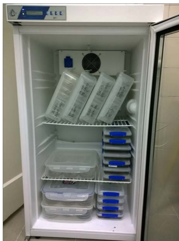
Fig. 89. Cultivation in a laboratory refrigerator at 19 °C in a comparative test of methods (top shelf – test tubes in an oblique position; lower shelves right – containers according to Hruška's method; lower shelves left – Petri dishes).
