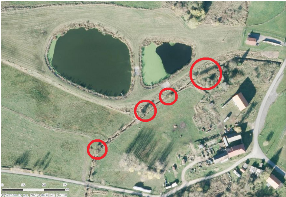
Fig. 262. Current state (2017) of overgrown fascine bundles with gravel (in red circles). Source: Mapy.cz, © Seznam.cz, a. s., © TopGis, s. r. o.
