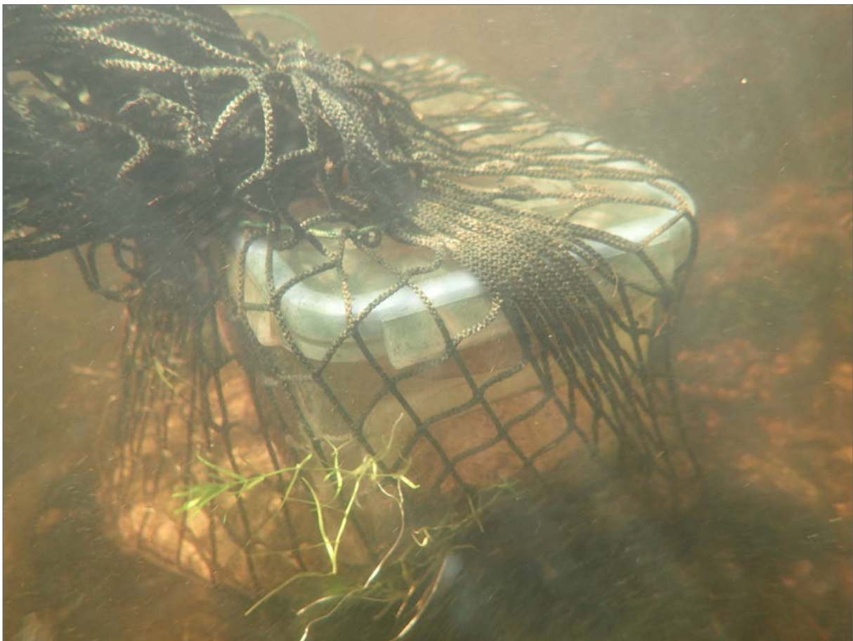
Fig. 57. A sand cage placed in the field immediately after installation (compare with a clogged cage in Figure 69).
