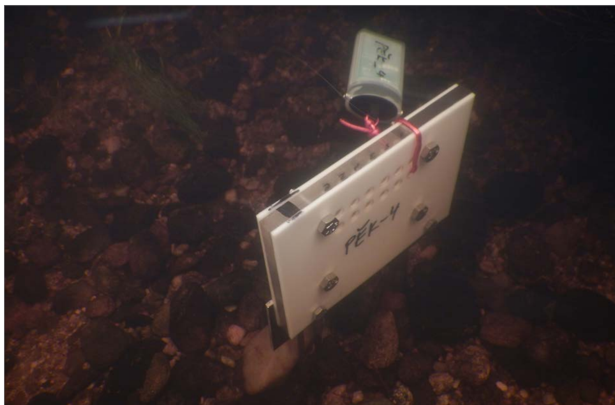
Fig. 66. Buddensiek bioindication plate installed on site with data logger (HOBO-Pendant, Onset) recording continually in one hour step temperature and light.
